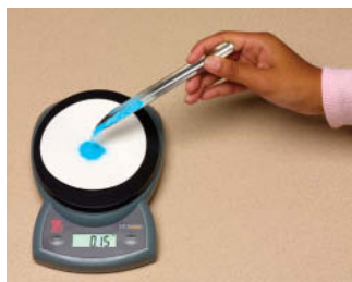
Tools for measuring mass: balance with weighing paper, spatula.
