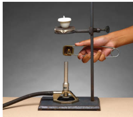
Tools for heating: Bunsen burner with striker, ring stand with utility clamp, and a triangle holding crucible.
