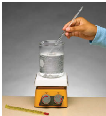
Tools for heating: Hot plate with beaker, boiling chips, and stirring rod, a thermometer.
