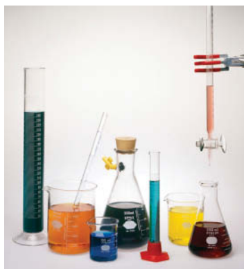
Tools for measuring volume: graduated cylinders, Erlenmeyer flask, burette attached to Erlenmeyer flask.
